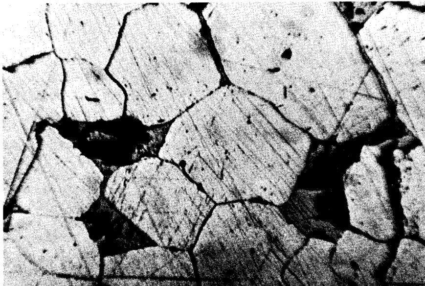
Figure 9. Photomicrograph of massive sulfide mineralization. Typical section of massive sulfide mineralization showing polygonal-shaped pyrite grains and interstitial chalcopyrite (light gray); pyrite grain shapes are probably the result of recrystallization. Pyrite grains about 0.5 mm. Reflected light.
