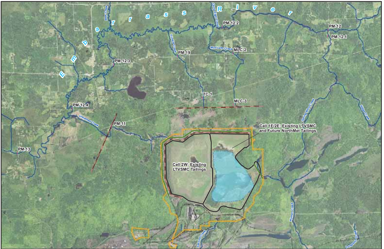
— Groundwater Evaluation Locations Plant Site — Groundwater Elevation Contours (feet) Existing Tailings Basin ! Surface Water Evaluation Locations Approximate Pond Area — Containment System ~ Stream/River 0 0.25 0.5 1 1.5 Miles Figure 5.2.2-13 Plant Site Contaminant Source Areas and Evaluation Locations NorthMet Mining Project and Land Exchange FEIS Minnesota November 2015
